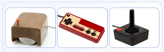
Pointing devices: Left: A 1968 prototype of the first mouse (Getty Images); 1983 Nintendo Famicom controller with D_Pad (Nintendo); (1977) Atari CX40 joystick (Atari)
