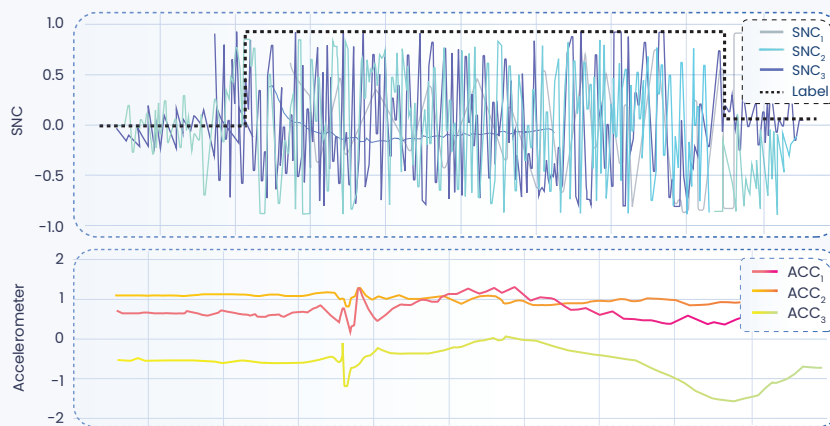
Figure 12: SNC and IMU signals for a swipe left gesture
